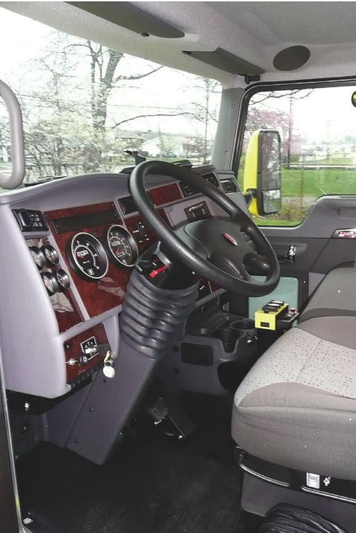
Big-rig-style dash and tall roof are pluses. Cab is narrow and short, and pedal placement cramps leg room, but drivers learn to live with it.
