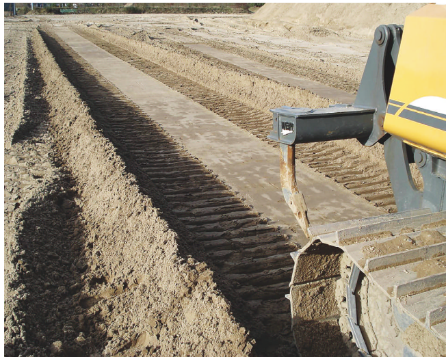
With the new 3D-MC 2 machine-control system, grading is possible with a dozer operating in second gear and, as shown here, even third gear.
