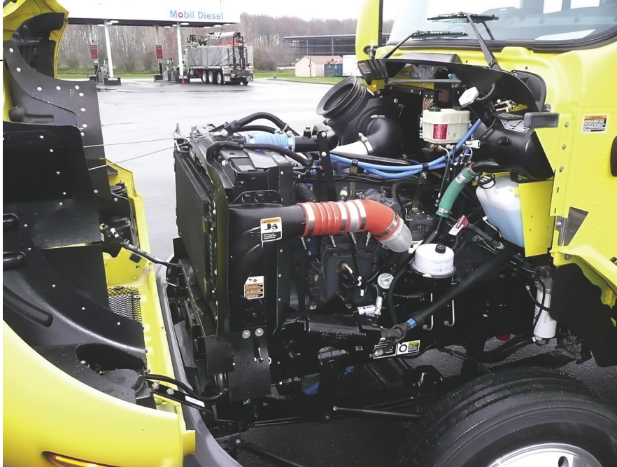
A Cummins-built Paccar PX-6 is gutsy. The hood is short, so space for the engine must come out of the cab’s lower front.
