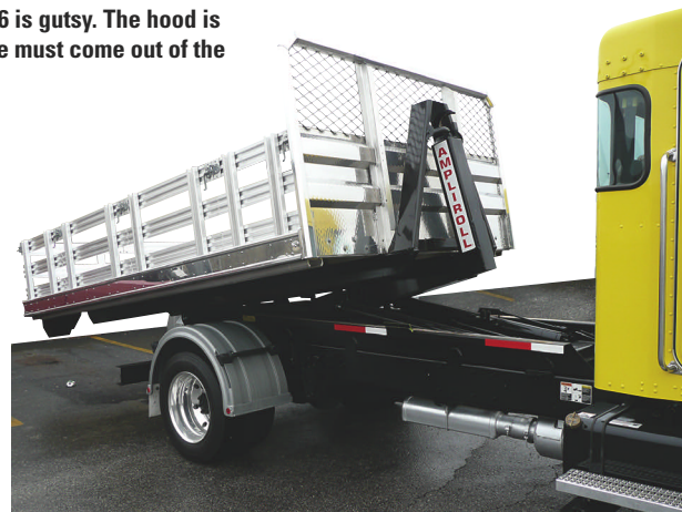
Ampliroll hook-lift mechanism can drop and snatch dump, flatbed, tank and service bodies, and more. It allows one truck to do multiple jobs.
